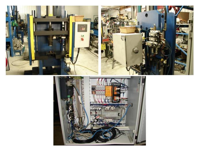
HYPERCYL ARIES ENGINEERING 20 ton Press, #HPS-20-6-.50-FH-LT, satellite cylinder and booster, 6" total stroke, .50" power stroke, flange mount, low voltage linear transducer, hydraulic hose assembly (1'-10') with dry-break style disconnect, output force @ 65 PSI: 25,210 lbs., prefilled and tested
