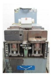
3" Eagle #EE double head vise & ram type tube end forming machine, capable of: expanding & reducing (C-Type tooling), vise & ram forming (E-Type tooling), double head – allows for (2) tooling sets to be set-up at once, accepts industry standard "drop-in" tooling
