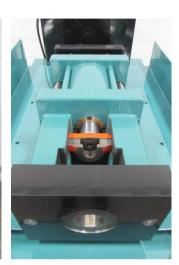
3" Eagle #IO Single Head Tube End Former, Includes Two Hand Cycle Start and Machine Mounted Operator Controls, Accepts Industry Standard "Drop-In" Quick Change IDOD type Tooling, Allen Bradley PLC and related controls
