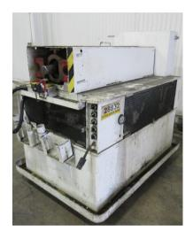
3" Eagle IO Single Head Tube End Forming Machine, Includes Two Hand Cycle Start and Machine Mounted Operator Controls, Accepts Industry Standard "Drop-In" Quick Change IDOD Type Tooling, Allen Bradley PLC and related controls
