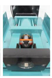
3" Eagle #IO Tube End Former, Capable of Expanding, Reducing, Tight Tolerance Sizing/Resizing on the ID & OD of Tubing, Custom Beading & Forming on the ID & OD of tubing, Includes Two Hand Cycle Start and Machine Mounted Operator Controls
