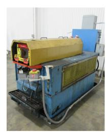
3" Eagle #HP90 single head vise and ram end forming machine, capable of expanding, reducing, custom beading & forming on inside & outside diameter of tubing, custom slotting, notching, piercing and sizing, accepts industry standard drop-in tooling, two hand cycle start switch, Allen Bradley PLC and related control system,
