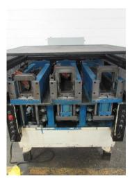
3" Eagle #EEE Triple Head Vise & Ram Tube End Former, (3) Forming Heads – allows for (3) independent forming operations all on common machine base, each with the following capabilities: Expanding / Reducing / Slotting / Notching / Piercing, Vise & Ram Forming – flaring & custom forming, Long forming operations using 12" stroke feature, Allan Bradley controls
