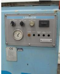
1-1/2" Langbow #TM38 twin head type tube bending machine,
