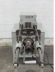
3-1/2" Coilco Extrupunch #12008 Tube Forming Machine
