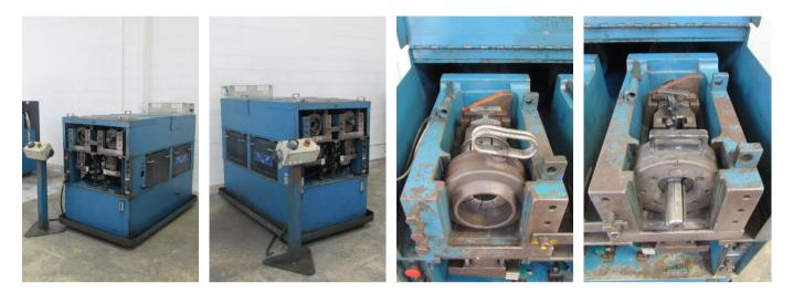
3" Eagle #EE double head vise & ram type tube end forming machine, capable of: expanding & reducing (C-Type tooling), vise & ram forming (E-Type tooling), double head – allows for (2) tooling sets to be set-up at once, accepts industry standard "drop-in" tooling
