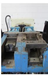
3" Custom #CE double head tube end former, capable of expanding, reducing, slotting, notching, piercing, vise & ram forming, machine mounted operator controls with PLC, accepts industry standard tooling.
