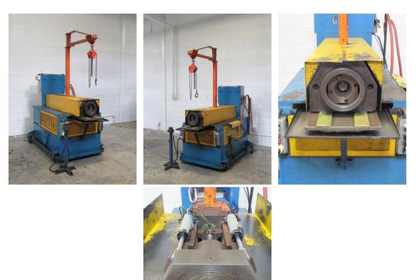
2" Eagle #LVR-100 hydraulic press tube end forming machine, capable of simultaneously pierce four rows of louvers in precent tube with one cycle, capable of working with tube up to 2" OD, machine mounted operator controls, jib crane mounted to machine for lifting in dies.
