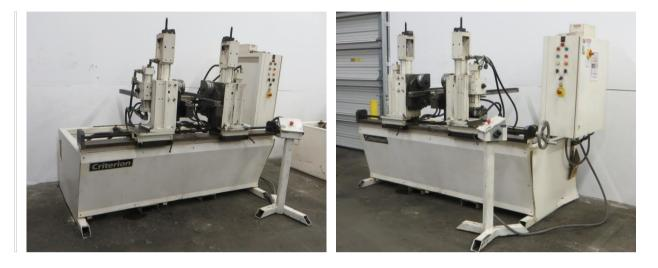
1-1/2" Criterion #26000 twin head hydraulic tube bending machine
