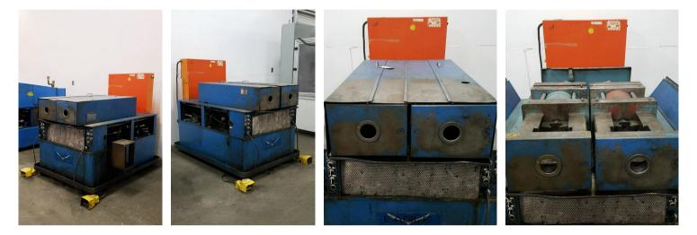
3" Eagle IOIO double head tube end forming and sizing machine
