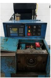
3" Eagle CNC IO-2000 high production tube end sizing machine
