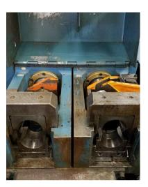
3" Eagle #EFEF double head vise & ram end forming machine with rotary tube feature
