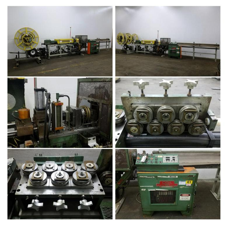
1-1/8" Burr Oak M5 high-production/high-precision round tube cut-off machine
