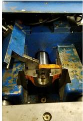
3" Eagle Eaton Leonard CNC IOC double head sizing & tube end forming machine
