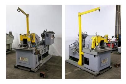
Torrington Vaill rotary tube end beading, forming & flaring machine
