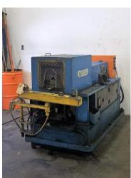
Eagle single head hydraulic operated ram form/spin flare/rotary form tube end forming machine
