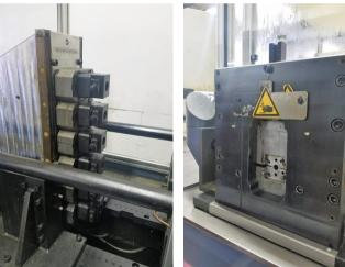
ROSENBERGER all electric 6-hit end former with automatic loader-used-
