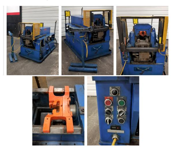
Eagle single head hydraulic operated ram form/spine flare/rotary form tube end forming machine Model: F
