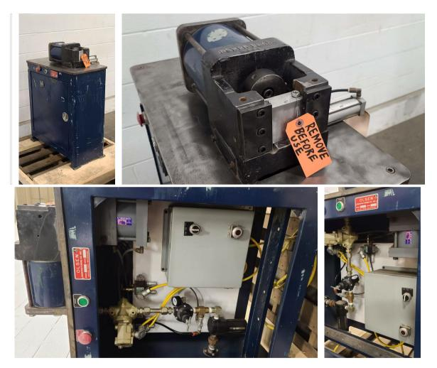
Olsen Bench top "Power Flare" semiautomatic double flaring machine Model: 20SA
