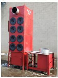
Micro-Air 4,000 cfm cartridge-type dust collection system
